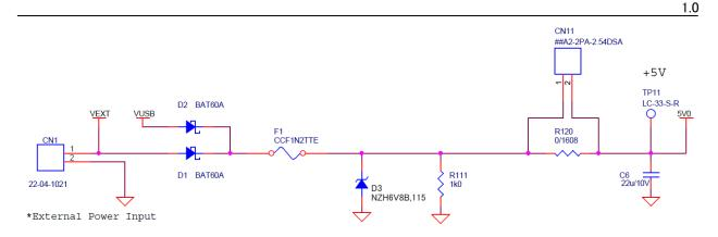
CN1 and + 5V from the USB connector are connected by diode OR as shown in the above circuit diagram.
