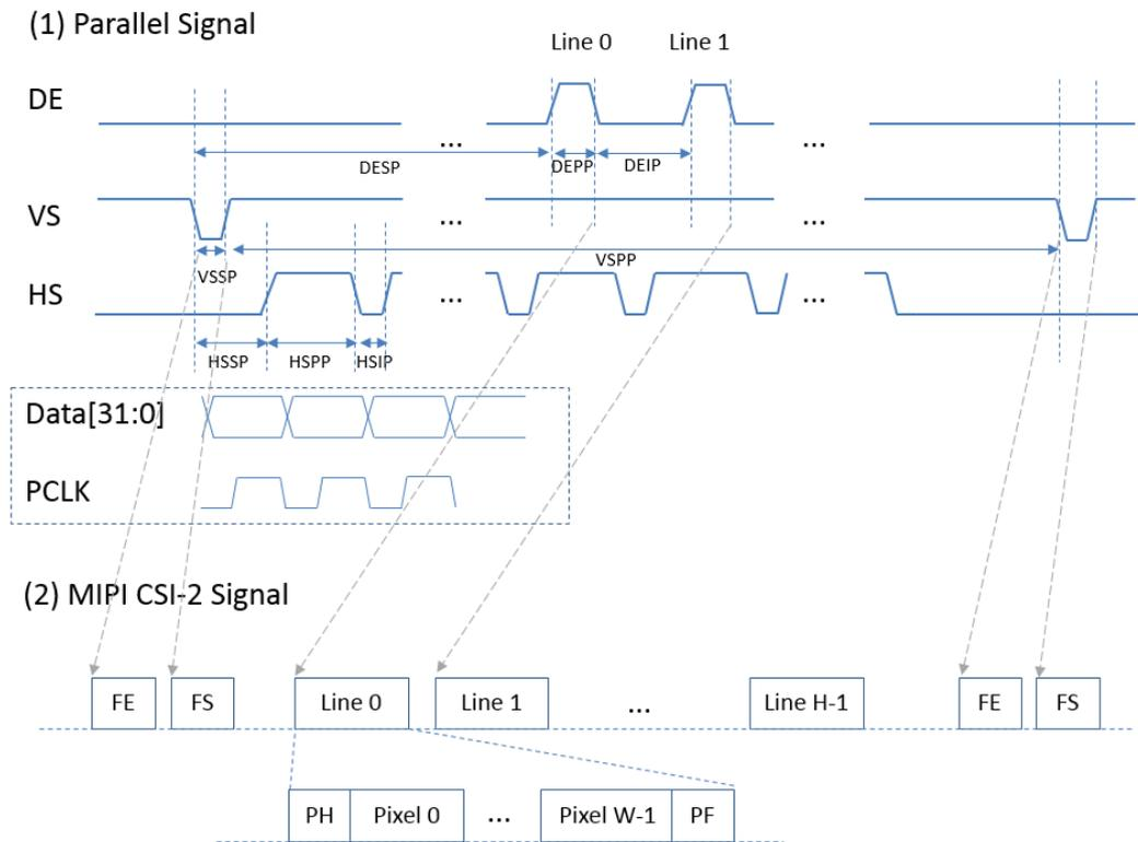
– FE: Frame End, FS: Frame Start, PH: Packet Header, PF: Packet Footer
