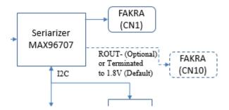
OUT1+ terminal of MAX96707 is output to CN1. OUT- terminal is connected to 1.8V through resistance R2 (49.9  $\Omega$ ). Normally it supports coaxial output using FAKRA connector.
